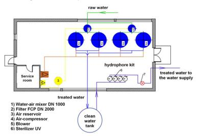
Fig. 1. Technological diagram of the Water Treatment Station in Drzenin
